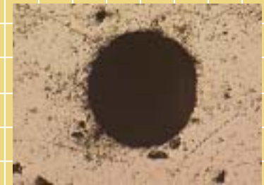
Optical fibers embedded in Al
