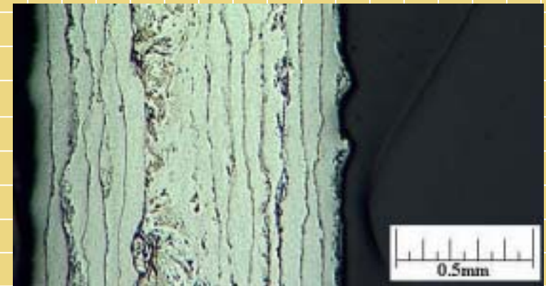
Fifteen layers of 0.001” Ti foil
