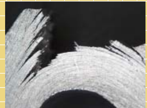
Charpy specimen made with UOC
